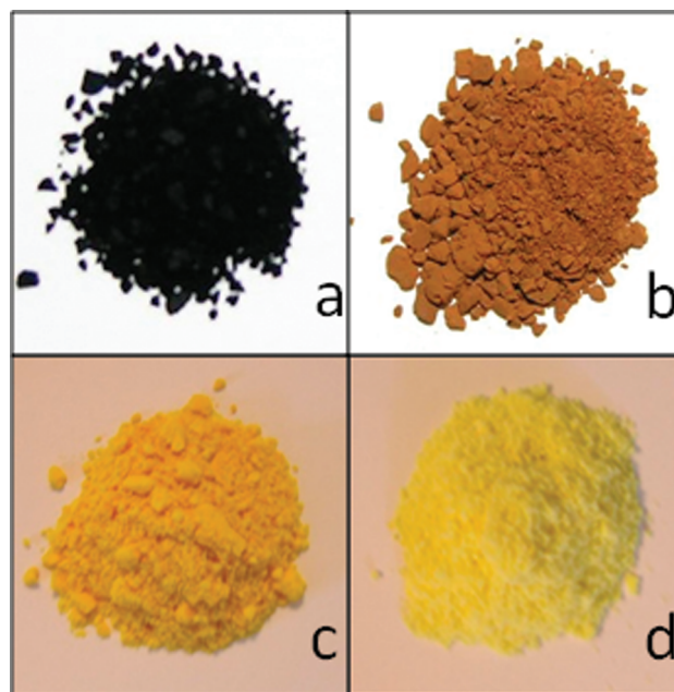
Figure 1. Color evolution from AF sample (a) and as a function of annealing treatments under air at 300 (A300C) (b), 350 (A350C) (c), and 400 °C (A400C) (d).
